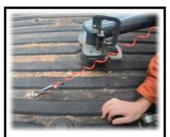
The most important thing about a trailer breakaway system is that the cable be attached to the towing vehicle
