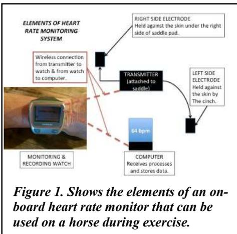
**Figure 1.** Shows the elements of an on-board heart rate monitor that can be used on a horse during exercise.
